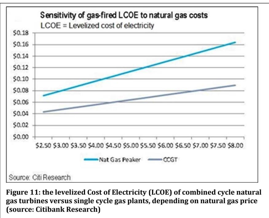
Figure 11: the levelized Cost of Electricity (LCOE) of combined cycle natural gas turbines versus single cycle gas plants, depending on natural gas price (source: Citibank Research)
