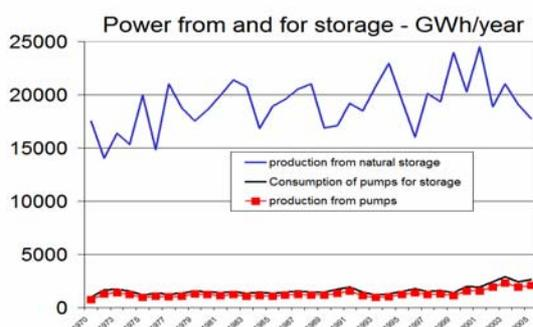
**Figure 59 Swiss hydro storage (blue) and pump storage production**
