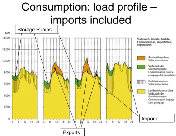
**Figure 13 daily electricity load curves - consumption**
