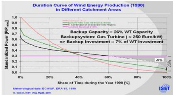
**Figure 47 Czisch: Duration Curve and Back-up needs**
