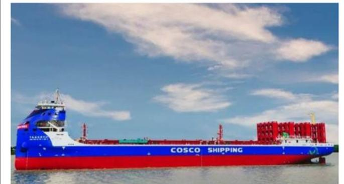
700 TEU containership is powered by containerized batteries that will be swapped out along the route (COSCO)
